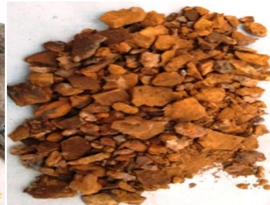
Figure 6 Şırnak Limonite Iron Ore Sand
