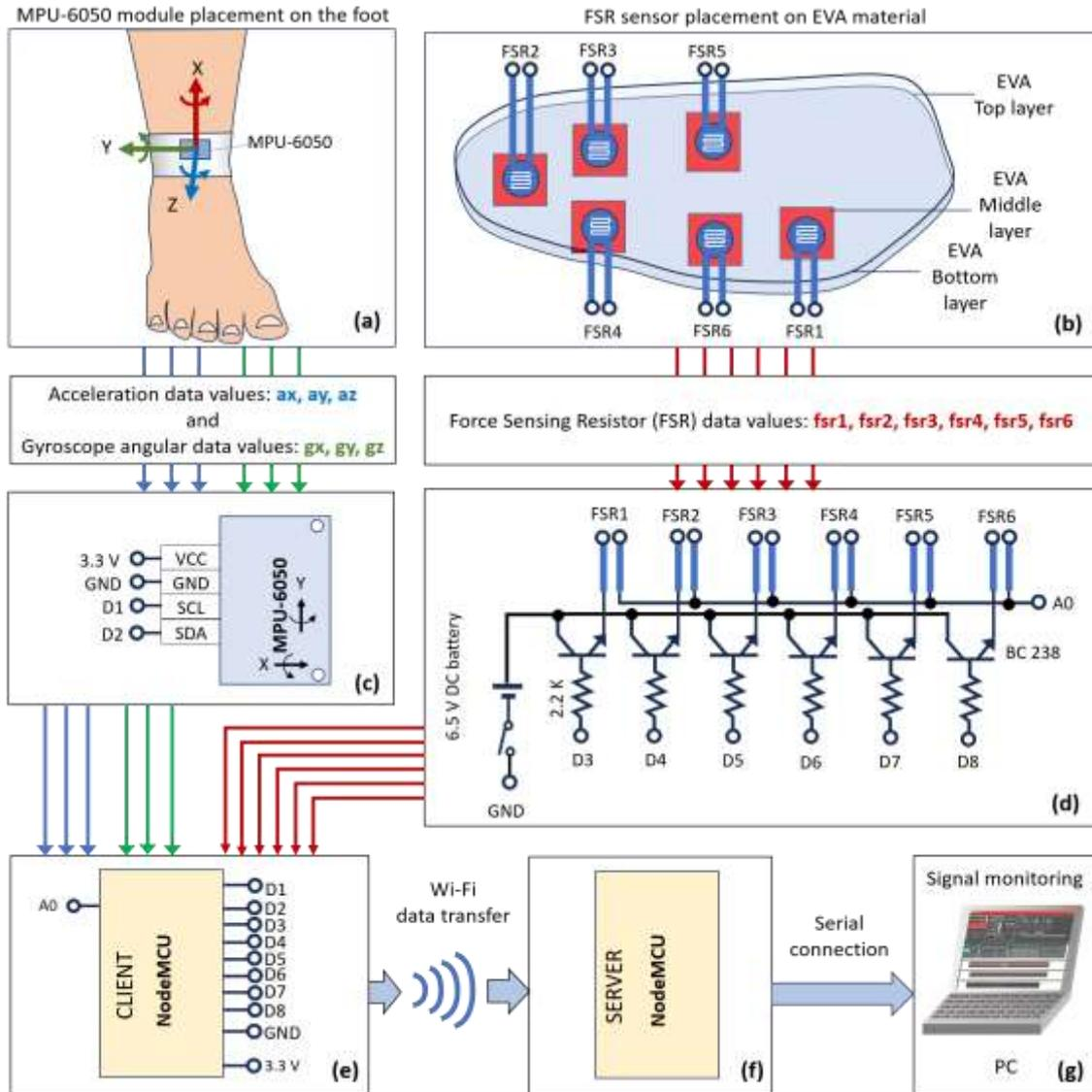
Figure 2: System design for transferring sensor data to the computer
