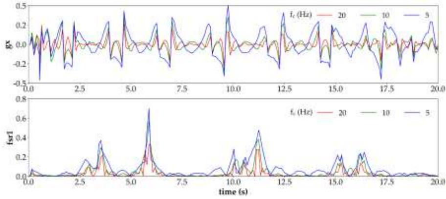
**Figure 10:** High-pass filter results of normalized gx angle and fsr1 force data are given for 5 Hz, 10 Hz and 20 Hz cut-off frequencies. The sampling rate is set to 100.
