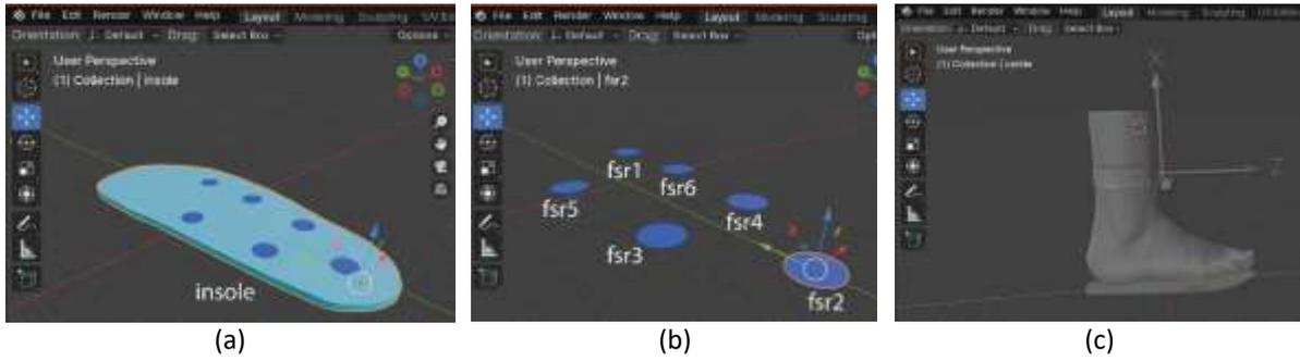
**Figure 6:** (a) 3D model of the insole (b) Cylinder models for showing the force of the FSR sensors (c) 3D foot model
