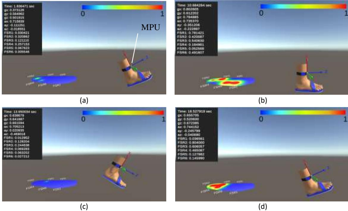
Figure 9: Heatmap based on walking step at (a) 1.83 s, (b) 10.68 s, (c) 13.65 s, and (d) 18.52 s
