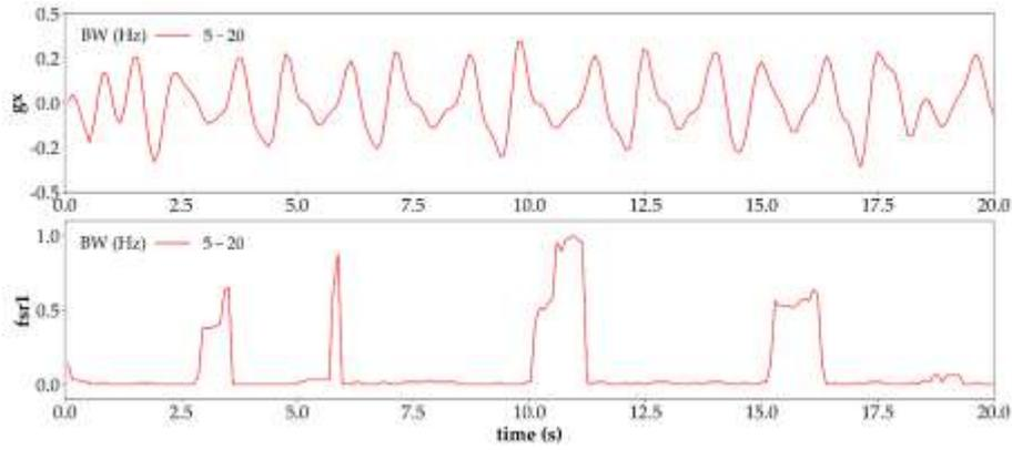
**Figure 11:** Band-pass filtering results of normalized gx angle and fsr1 force data are given for 5-20 Hz bandwidth (BW). The sampling rate is set to 100.
