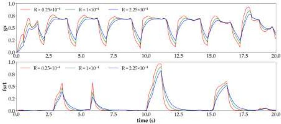
**Figure 12:** Kalman filtering results of normalized gx angle and fsr1 force data are given for the measurement variance estimation R values of  $0.25 \times 10^{-4}$ ,  $1 \times 10^{-4}$  and  $2.25 \times 10^{-4}$ . Q variance value is used as  $1 \times 10^{-4}$ .
