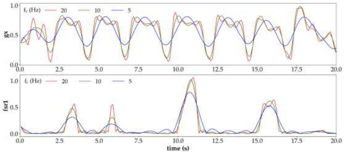
Figure 5: Low-pass filtered signals for gx angle and fsr1 force data for cut-off frequencies of 20 Hz, 10 Hz and 5 Hz.
