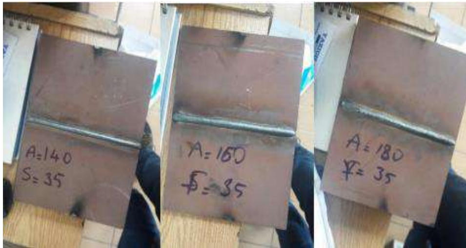
Figure 1. Welded plates obtained at different welding currents
