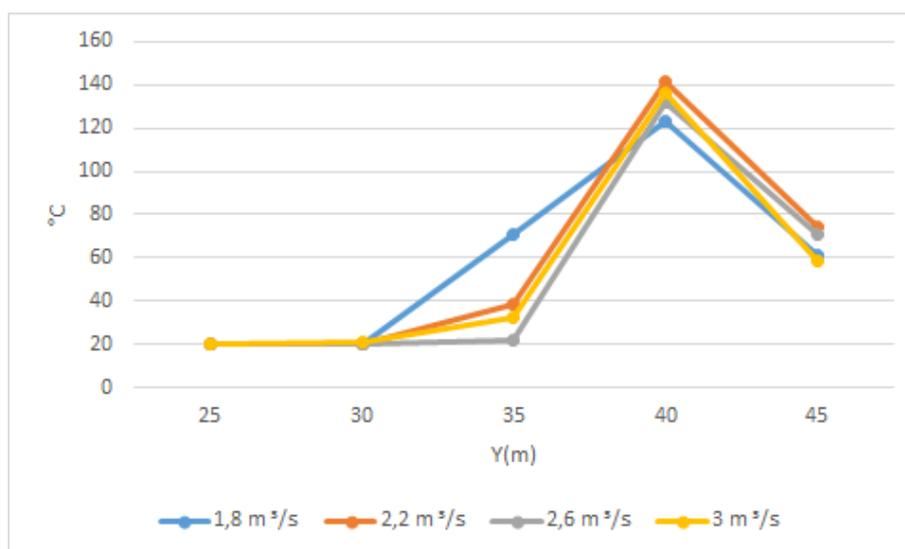
**Figure 7.** For HRR=500 kW,  $x=25$  m,  $z=2.35$  m, and  $t = 360$  s change of temperature with fan flow along y axis
