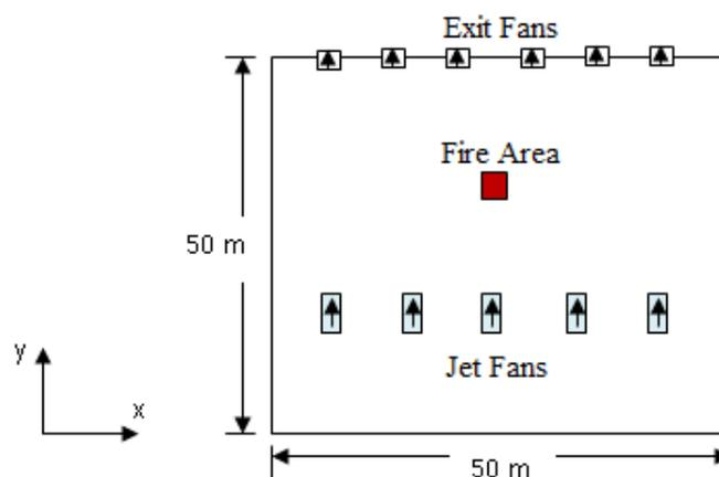
**Figure 1.** Schematic representation of top view of problem geometry**2.1. Problem equations**
