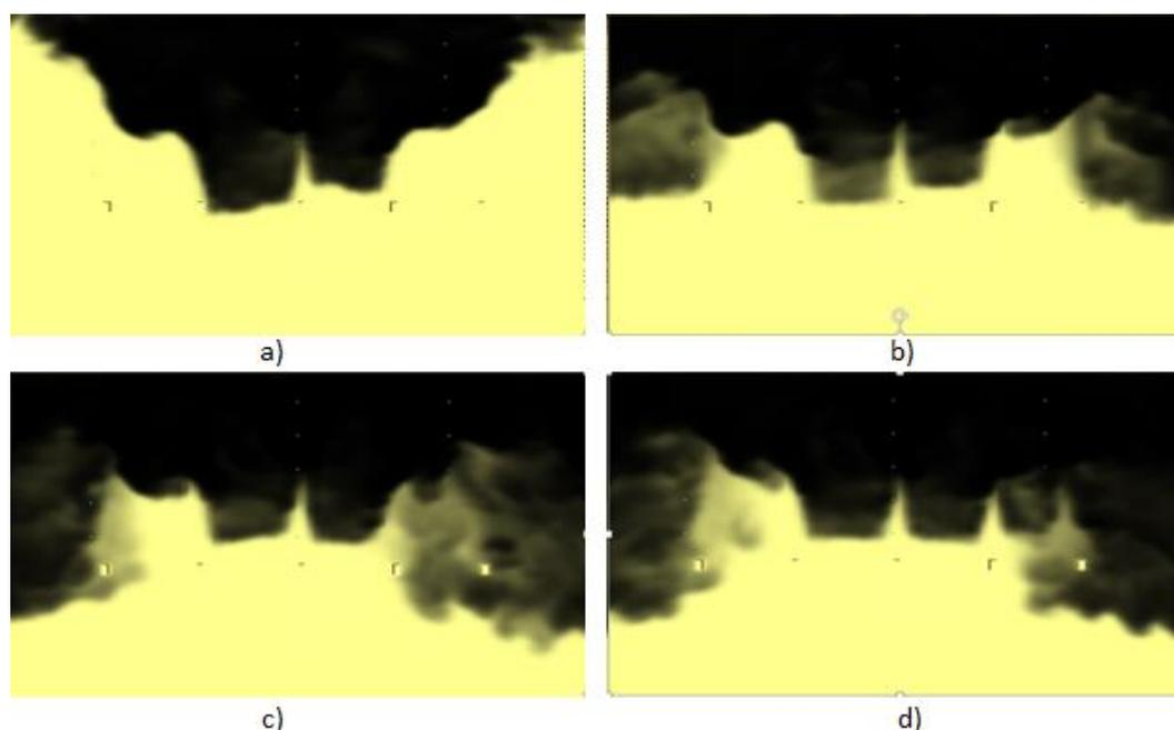
**Figure 2.** For HRR=1000 kW,  $z=1.62$  m, and fan flow  $3 \text{ m}^3/\text{s}$ , smoke distribution during different time frames of fire a)  $t=30$  s, b)  $t=140$  s, c)  $t=250$  s and d)  $t=360$  s
