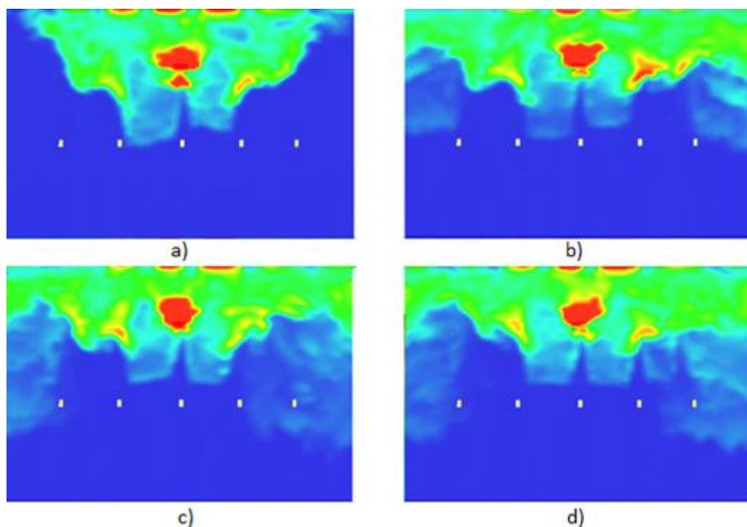
**Figure 3.** For HRR=1000 kW,  $z=1.62$  m, and fan flow  $3 \text{ m}^3/\text{s}$ , temperature distribution during different time frames of fire a)  $t=30$  s, b)  $t=140$  s, c)  $t=250$  s and d)  $t=360$  s
