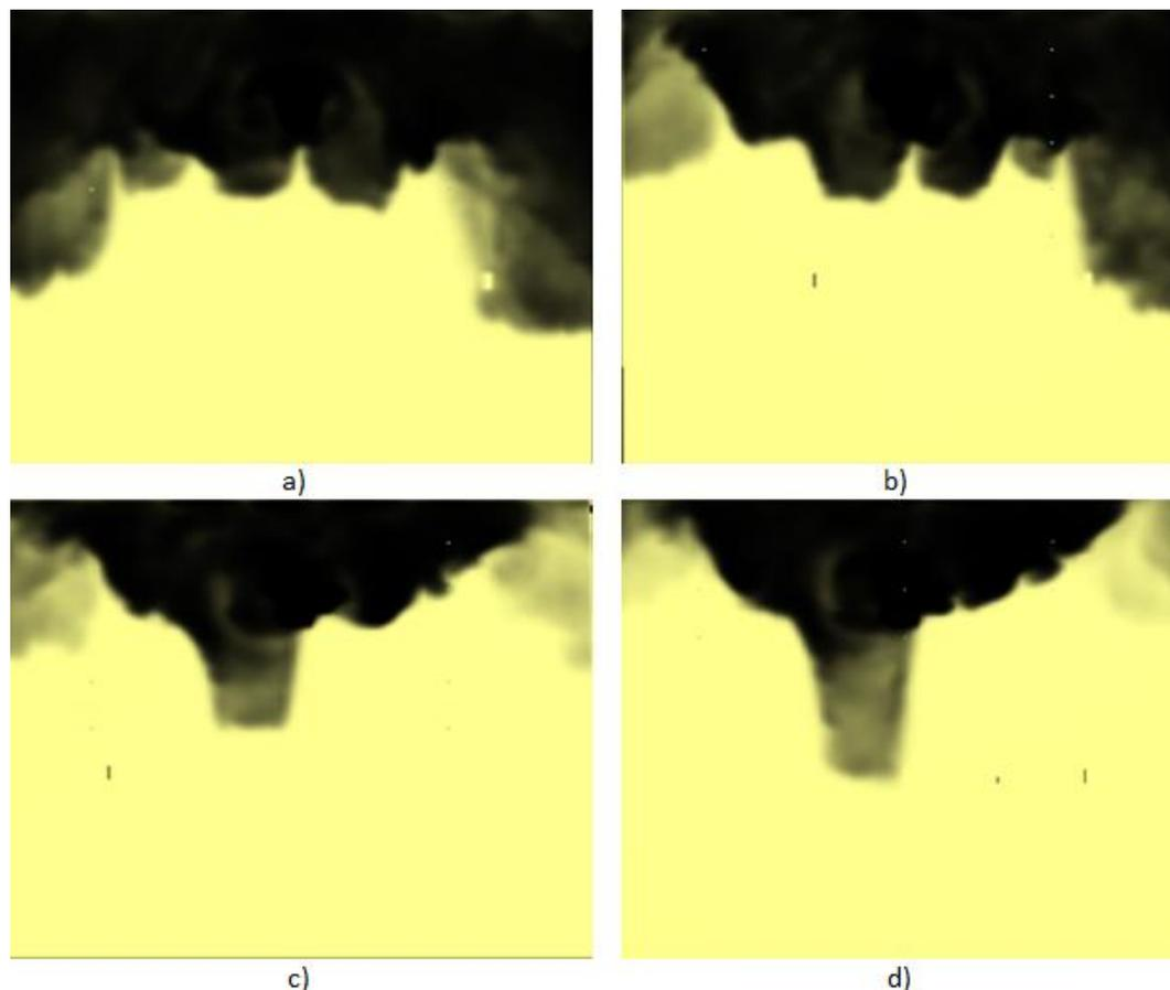
**Figure 5.** For HRR=500 kW,  $z=1.62$  m, and  $t=360$  s smoke distribution for different fan flows, a) 1.8 m<sup>3</sup>/s, b) 2.2 m<sup>3</sup>/s, c) 2.6 m<sup>3</sup>/s and d) 3 m<sup>3</sup>/s
