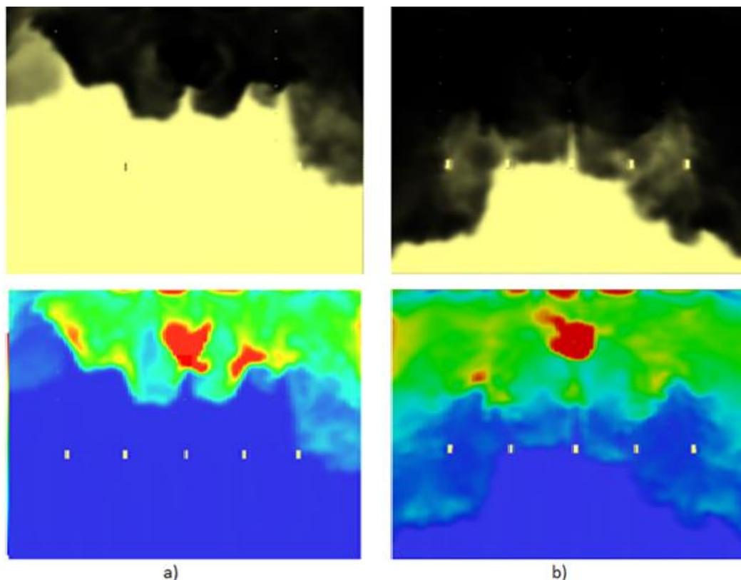
**Figure 6.** For fan flow  $2.2 \text{ m}^3/\text{s}$ ,  $z=1.62 \text{ m}$ , and  $t=360 \text{ s}$ , smoke and temperature distribution for fires with different heat release ratio a) HRR=500 kW, b) HRR=1000 kW
