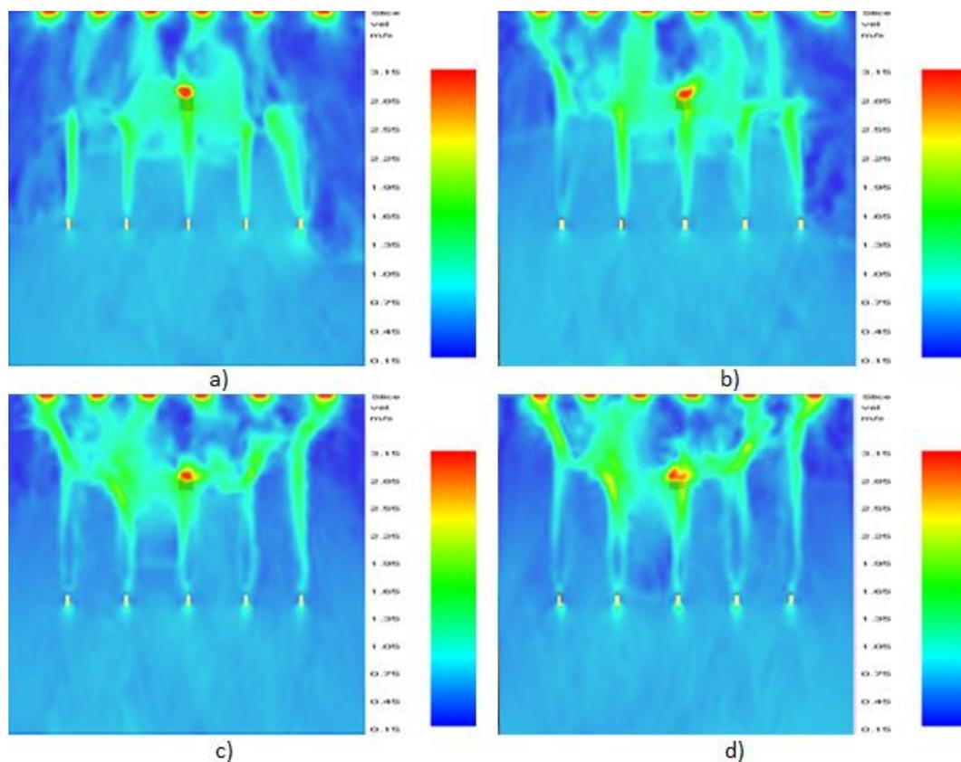
**Figure 4.** For HRR=500 kW,  $z=1.62$  m, and  $t=360$  s speed distribution for different fan flows, a)  $1.8 \text{ m}^3/\text{s}$ , b)  $2.2 \text{ m}^3/\text{s}$ , c)  $2.6 \text{ m}^3/\text{s}$  and d)  $3 \text{ m}^3/\text{s}$
