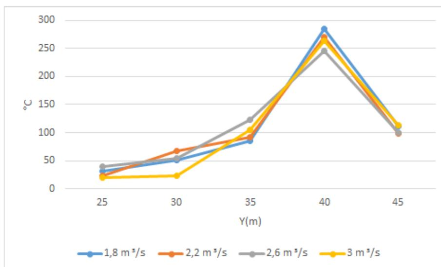
**Figure 8.** For HRR=1000 kW,  $x=25$  m,  $z=2.35$  m, and  $t = 360$  s change of temperature with fan flow along y axis
