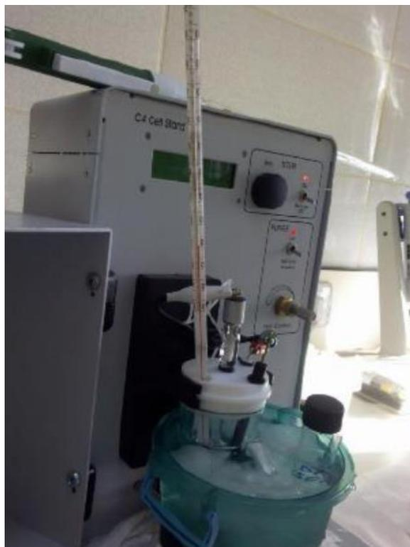
**Picture 2.** The image of the cell in a cold water bath in the determination of dopamine with MoS<sub>2</sub>(1)/GCE
